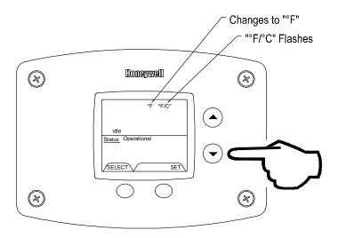
Step 4: Press "Set" button to confirm °F or °C format. °F/°C will stop flashing
